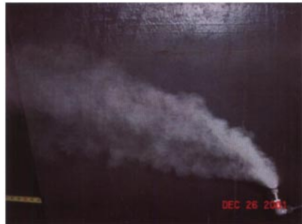
Fig. 10 90 deg orientation of a fog nozzle in the wind tunnel; airflow velocity is 4 m/s (800 ft/min), operating pressure is 138 barg (2000 psig)
