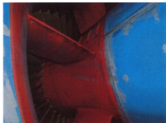
Fig. 17 Intake cone and struts at an axial compressor inlet
