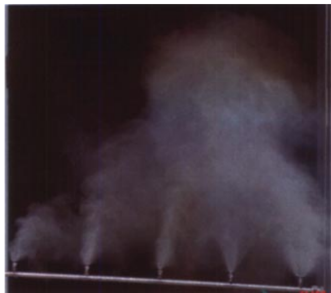
Fig. 5 Various impaction-pin nozzles, from 147-micron (on right) to 457-micron orifice diameter (left), operating pressure 138 barg
