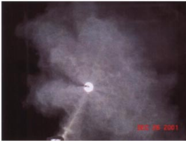
Fig. 11 Counterflow orientation of a fog nozzle in the wind tunnel; airflow velocity is 4 m/s (800 ft/min), operating pressure is 138 barg (2000 psig)
