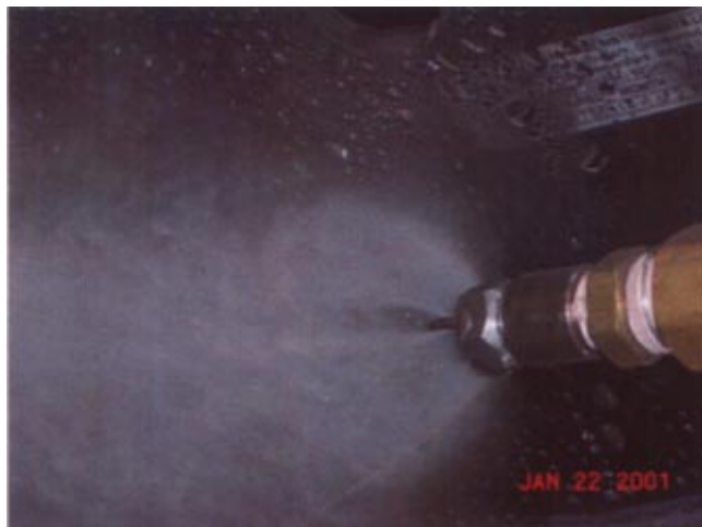
Fig. 6 Impaction-pin nozzle showing small shading effect from impaction pin
