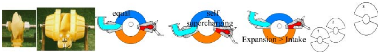
Fig. 1 (Left) stereolithography model of basic configuration; (center) one-disk compression-ratio variations; (right) multidisk shaft arrangement and compression-ratio variations
