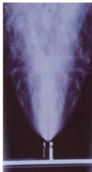
Fig. 3 Fog from an impaction pin-fogging nozzle operating at 2000 psig (138 barg)
