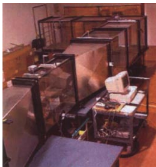
Fig. 4 Experimental wind tunnel (10.5 m long, 25 m/sec) used to study droplet kinetics and thermodynamics. This wind tunnel provides dynamic similarity to gas turbine inlet ducts.
