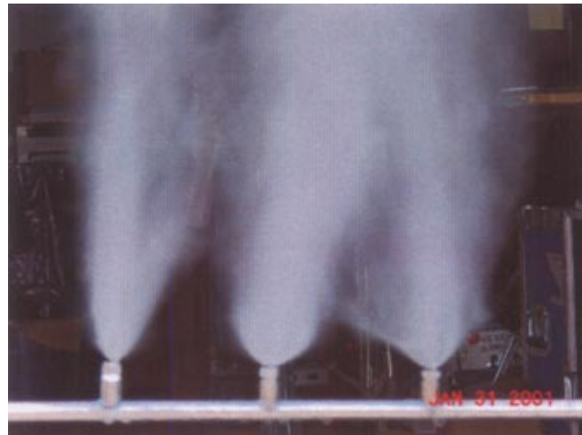
Fig. 4 Visual plume shape of different makes of impaction-pin nozzles at an operating pressure of 138 barg (2000 psig). Mee nozzle (152 micron orifice, 316 stainless steel construction) in the center
