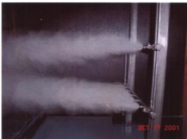
Fig. 12 Side view of nozzle array; airflow velocity is 4 m/s (800 ft/min) operating pressure is 138 barg (2000 psig)
