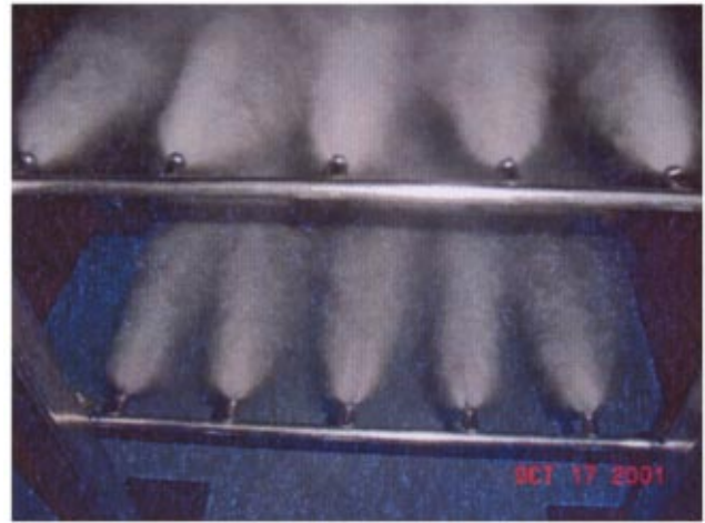
Fig. 13 Face view of nozzle array; airflow velocity is 4 m/s (800 ft/min), operating pressure is 138 barg (2000 psig)
